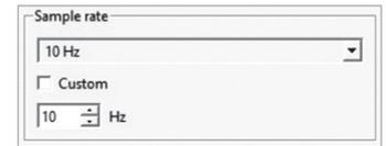
And, most importantly, let's see what the nature of this consumption is. First of all, we will select the sample rate- the frequency with which we will measure the current consumption value. Let it be 100 Hz. Use the dropdown list to select the desired value.
