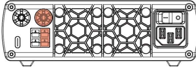
The loads can be connected also to Anderson Powerpole® connectors at the rear panel. There are additional connectors at the rear panel of the power supply:
