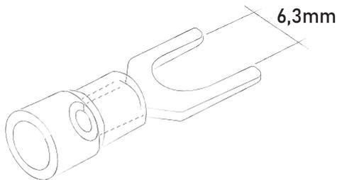
It is recommended to connect the load to the binding posts by Fork spade terminals.
