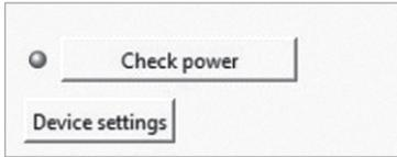
The REAMP companion software allows you to configure the device to make it convenient for you to work with it. To go to customization mode, click the Device Settings button.
