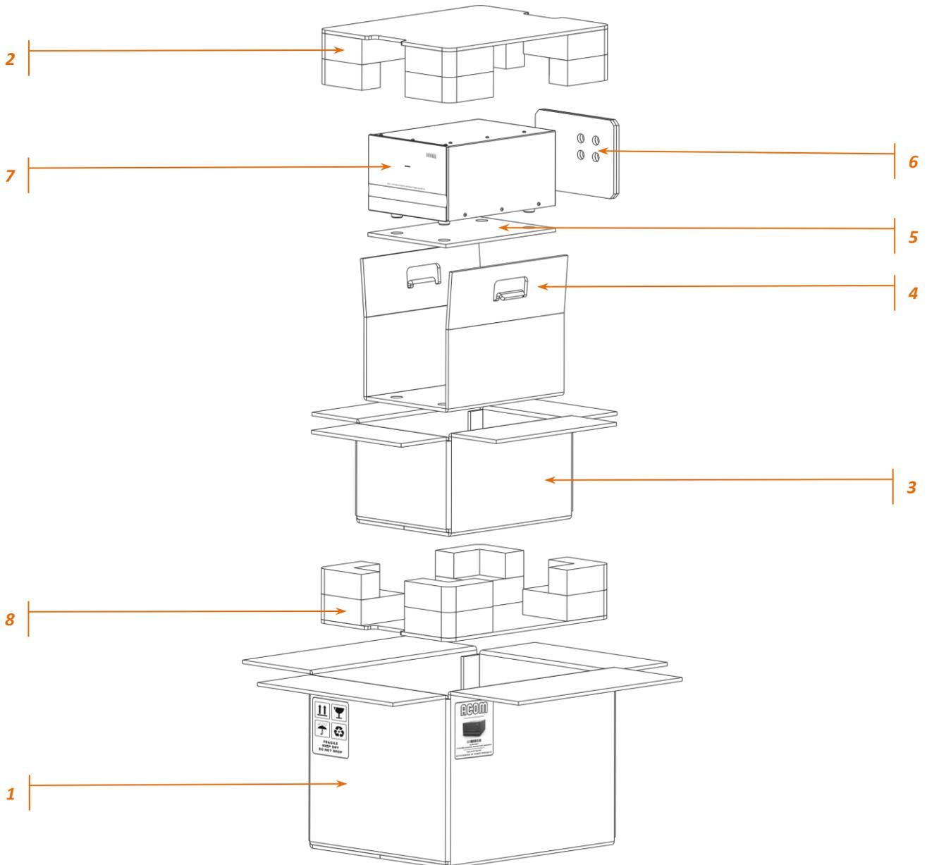
Figure 2-2 | ACOM 06AT packaged in a cardboard box
