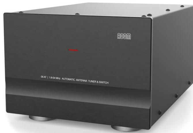
ACOM 06AT automatically selects one of four available antenna outputs (as assigned in bands by the operator) and matches the impedance of the chosen antenna output by transforming it to 50 Ohm with SWR below 1.5:1 at the tuner input (typically below 1.3), providing an optimum load impedance for the amplifier.
