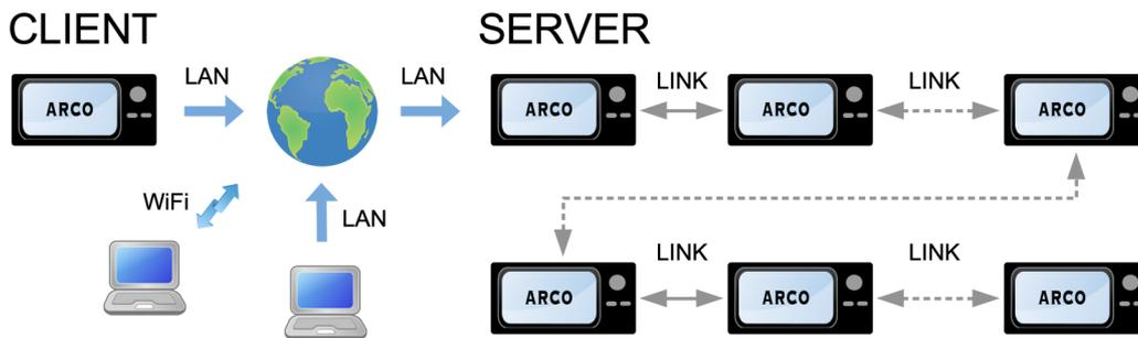
For Internet remote control from the computer we recommend to use PstRotatorAz program by YO3DMU. It can connect ARCO box directly providing necessary interface between logger on your computer and remotely located rotator controlled by ARCO. No computer is required on rotator side.
