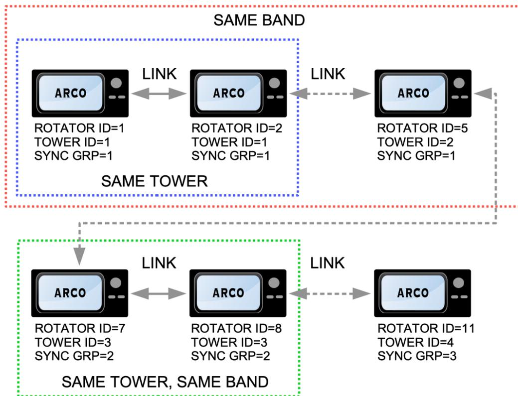
**COUNTER TO ROTATOR ID:** Enables counter rotation to the specified ARCO controller present on the LINK bus. This is a special setting for the ARCO controlled rotator which is installed over another rotator or on a rotating tower also controlled by own ARCO controller. COUNTER TO ID number specifies ROTATOR ID number of that controller. This function works always in pairs and requires SYNC ENABLE option to be enabled in menu and turned ON on the main screen.
