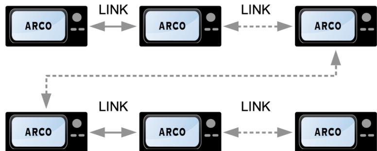
**LINK ENABLE:** Enables local remote control of the ARCO controller from another ARCO controller present on the LINK bus. Each ARCO MUST HAVE unique ROTATOR ID number.
